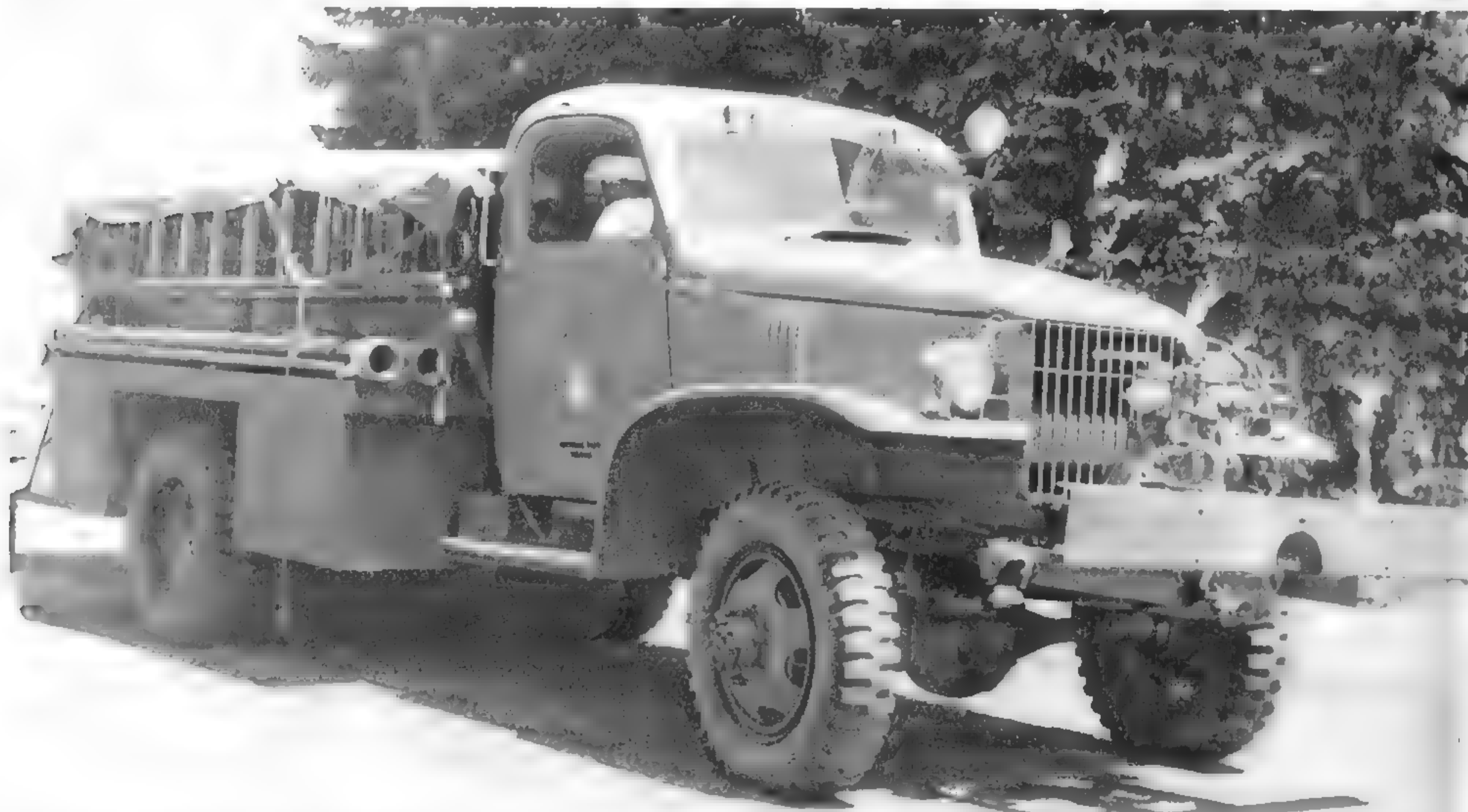
Shown here is a Class 525 fire truck, which was built on the Chevrolet Chassis. This particular truck was photographed after it had been transferred to the U.S. Department of Interior, but appears to be unchanged from its military days. The large fire pump mounted behind the front bumper was not required by the foam truck. (Photo from the Richard Adelman Collection)
